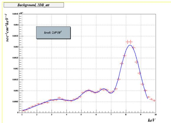
Fig. 5. Micromegas detector background data after cuts. The level achieved is  $2.0 \cdot 10^{-5}$  events/keV/cm<sup>2</sup>/sec between 1-10 keV.
